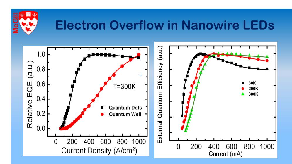
The presence of electron overflow leads to efficiency droop for the quantum dot emission at relatively high injection conditions.
