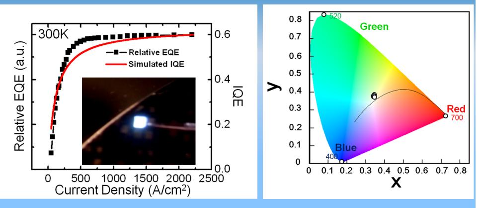
InGaN/GaN dot-in-a-wire white LEDs can exhibit a record high internal quantum efficiency (~ 60%) and are virtually free of efficiency droop for injection current density up to ~ 2,200 A/cm<sup>2</sup> at room temperature.
