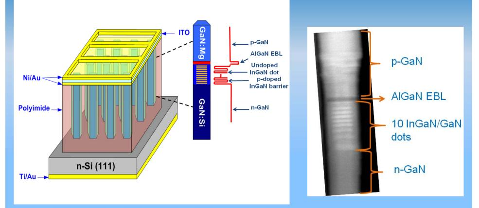
AIGaN electron blocking layer and p-type modulation doping are incorporated in the device active region to reduce electron overflow and to enhance the hole transport, respectively.
