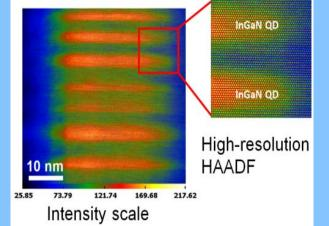
Catalyst-free InGaN/GaN dot-in-awire heterostructures are grown by molecular beam epitaxy on Si(111) substrates.
