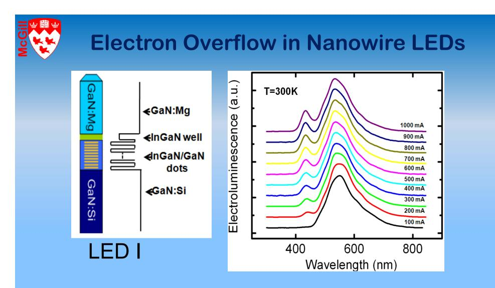
With the use of a test well (λ ~ 430 nm) between the quantum dot active region (λ ~ 550 nm) and the p-GaN, electron overflow is clearly measured in nanowire LEDs.
